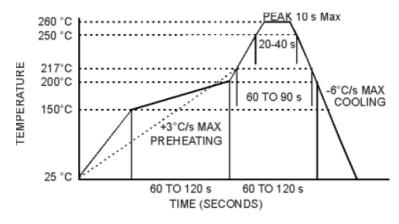
The device may be reflowed once. Reflowing upside down is not allowed. NO CLEAN assembly is recommended
